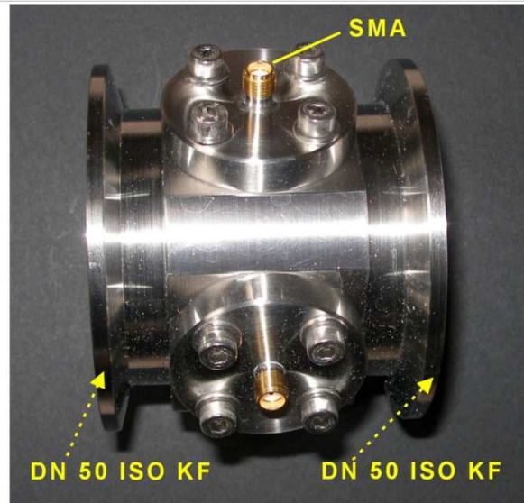
Beam Position Monitor in 50 Ohms Geometry
