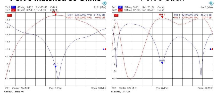
We can clearly see that we have matched and exceeded the manufacturer results of -31dB in the S11 and -0.150dB of S21
