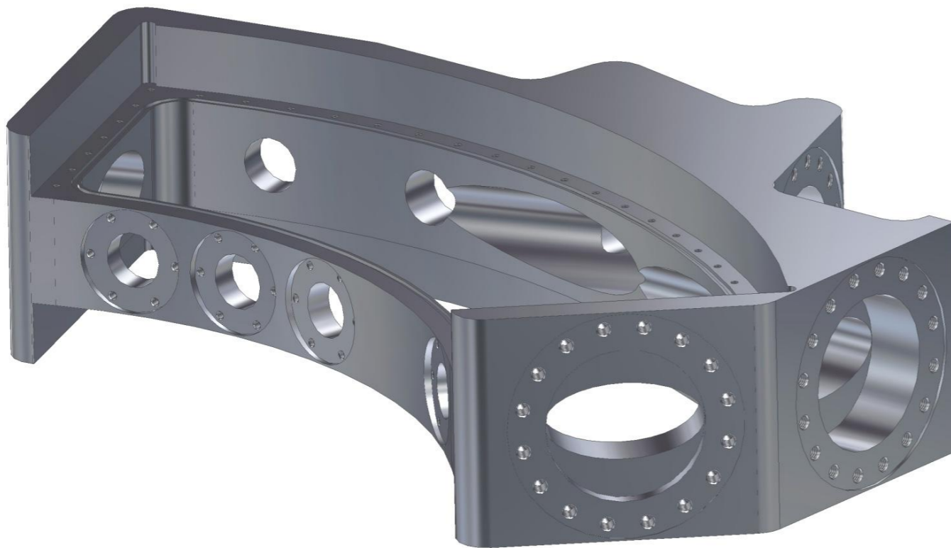
3 window ports for laser entry
