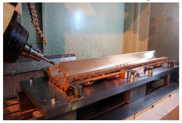
One major vane has been completed and awaits inspection before proceeding to finish the remaining pieces of RFQ section 1. The CMM is now fully operational and the inspection document is complete. The document allows measurements to be cross-referenced back to the original vane modulations spreadsheet. In the meantime the machining of RFQ section 2 has progressed.
