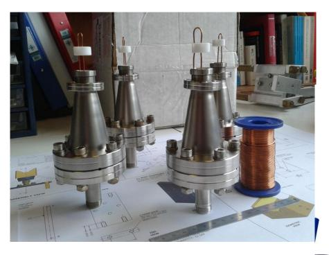
Four RFQ pick-ups have been built that will be used during the beadpull tests and for feedback to the RFQ tuning system.
