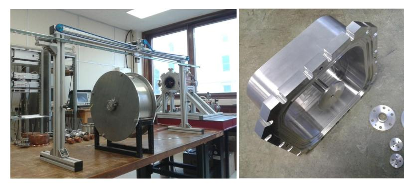
The bead-pull apparatus has been extended to cover one RFQ section and the end flange assemblies for the flat vane RFQ regions are complete. The bead-pull system will be tested inside the pill-box cavity and will then be ready for transport to RAL.
