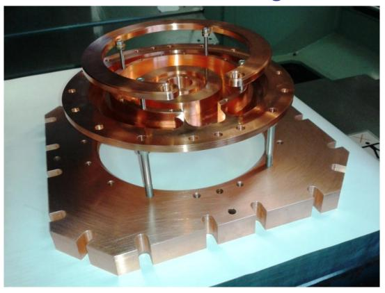
Both end flange assemblies have also been vacuum brazed, and have been tested for water leaks and vacuum leaks. They, along with the tuners are awaiting vacuum testing to 10<sup>-6</sup> mbar.
