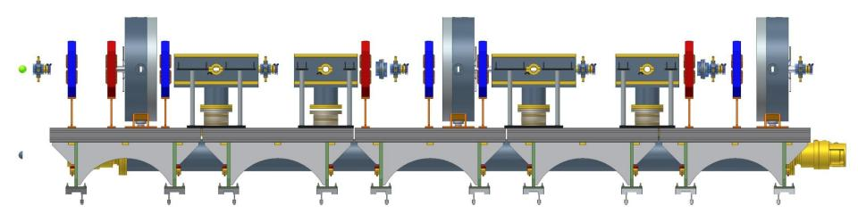
DN160CF vertical vacuum tubes now part of chopper and chopper beam dump bases. This would allow the vacuum manifold build to proceed prior to knowing vessel depths.
