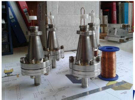
Four RFQ pick-ups have been built. Two will be used during the bead-pull tests. One pick-up per RFQ section is available for the feedback system.
