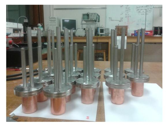
Sixteen tuners for RFQ section 1 have returned from the vacuum brazing company and have been vacuum tested to 10<sup>-3</sup> mbar. Vacuum components are on order to allow testing to 10<sup>-6</sup> mbar.
