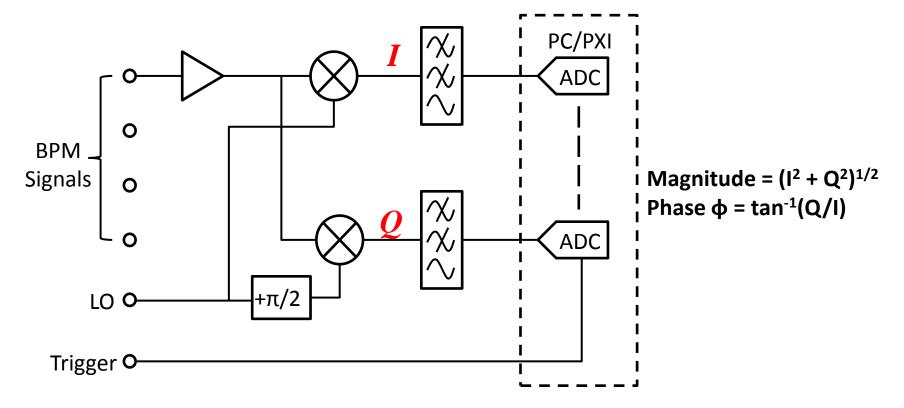
Can create both I and Q in electronics and use two digitizer channels to sample. Accurate but inefficient use of digitizer. I/Q results more accurate than I-only
