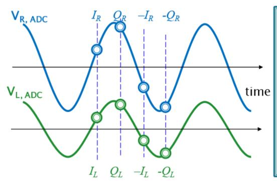
$$\Delta x = \frac{M_R \text{-}M_L}{M_R \text{+}M_L \text{+}M_U \text{+}M_D}$$
