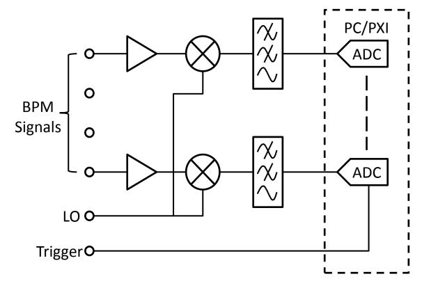
Each electrode is mixed to an IF of 10MHz, sampled at 50MS/s, split into 'segments', max and min of each segment found, maxes and mins meaned, difference/sum position calculated
