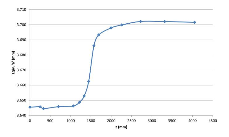
Including all the known effects such as modulation, tuning grooves, vacuum ports, fixed tuners etc the RFQ field from CST is reasonably flat (+/- 2%) with all the tuners in the 'flush' position.
