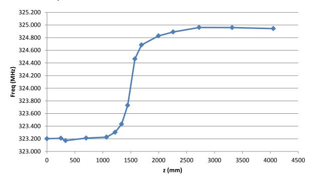
The frequency shift is compensated by tuning grooves in sections 2, 3 & 4 but if the grooves are to be included in the model the effect of the modulation has to be included too. Meshing limitations mean it is unfeasible to actually include the modulation in the model.
