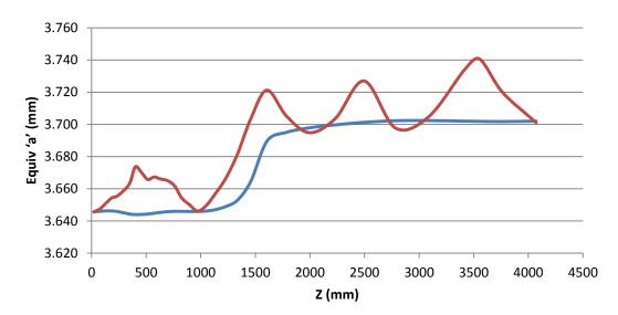
Equivalent smooth unmodulated vane aperture including the effect of modulation and errors.
