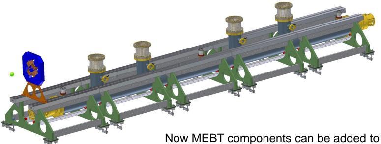
the frames. Here the first quadrupole has been positioned on the T-slot rails. It's position can be coarsly made by tape measure before final positioning by Adrian Hooper and team.
