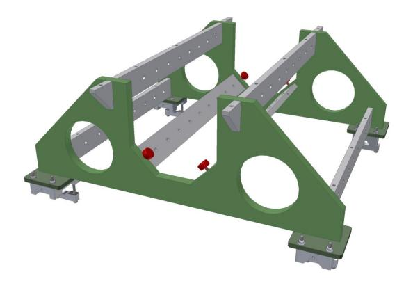
After the assembly has been welded the feet and top will be skimmed to gain the required flatness.
