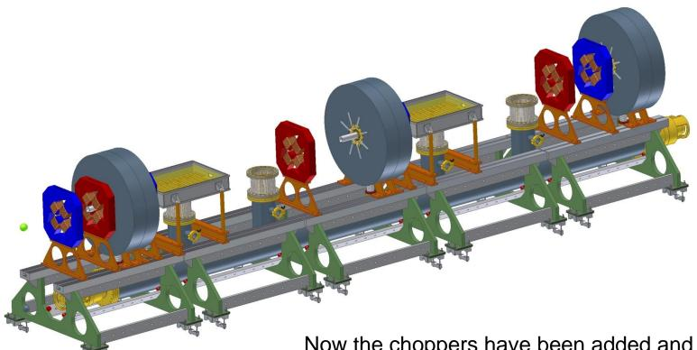
Now the choppers have been added and can be secured to the vacuum manifold. Note that the downstream slow chopper has been shown as a meander type just for ease of CAD modelling.
