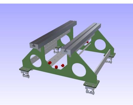
The MEBT support frame is a welded mild steel assembly that is approximately one metre long. It's transverse U-shaped profile accepts the vacuum manifold. The lack of high level cross bracing allows for any MEBT component spacing and hence will accommodate either the 3 or the 4 rebunching cavity lattice.
