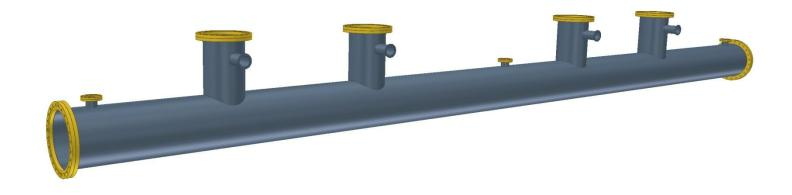
Next the DN200CF, DN160CF, DN40CF flanges are welded into position. I have also shown 4 x KF40 ports below the DN160CF flanges that could be used for vacuum measurement.
