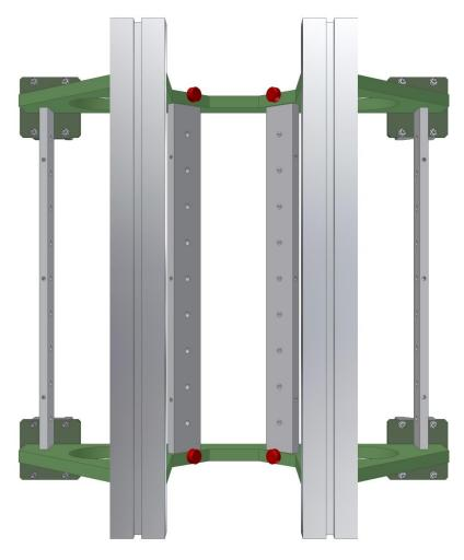
The plan view shows the off-the-shelf adjustable rubber feet that the vacuum manifold will sit on.
