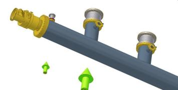
In total 558kg will push the manifold upwards towards the MEBT components. Because the MEBT components are secured to the rails the effect would be to compress the bellows.
