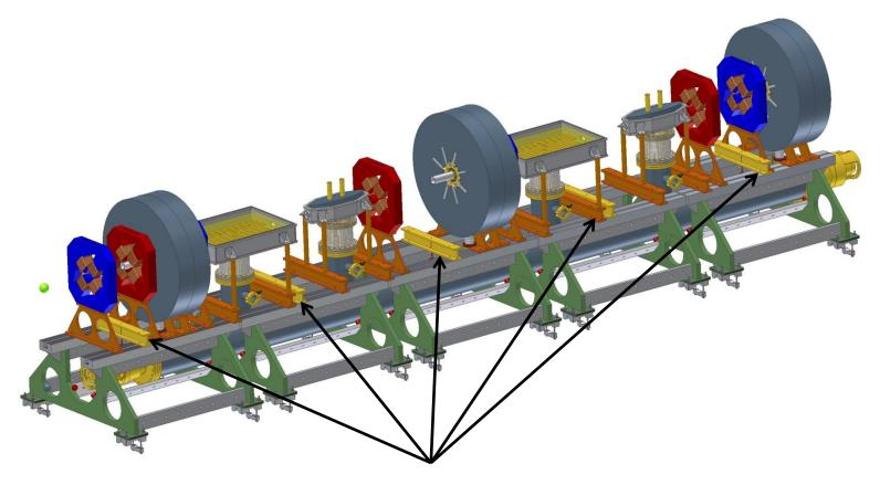
Five transverse beams are shown here in yellow. On their underside they will have a simple, off-the-shelf threaded rubber foot that can be wound down until it contacts the manifold.
