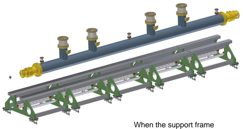
chain is complete the vacuum manifold can be lowered into position.
