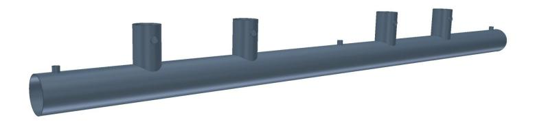
At its core the MEBT vacuum manifold is a long (~4.5m) DN200CF stainless steel tube. To one side of this tube are welded 4 x DN160CF tubes which align with the choppers and chopper beam dumps and 3 x DN40CF tubes which align with the rebunching cavities.
