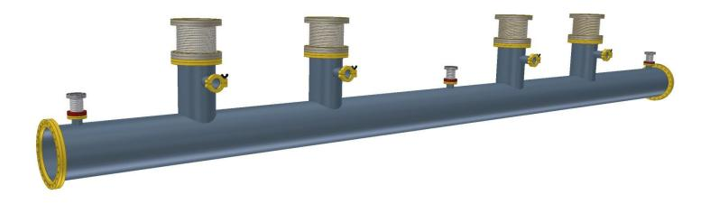
Next the bellows and KF40 flange blanks are fitted into position. Either the bellows are the manifold flanges will need to be rotatable. The bellows to be used are the hydro-formed type. They are cheaper and than the edge-welded type but will offer sufficient movement to compensate for manifold to MEBT component misalignment.
