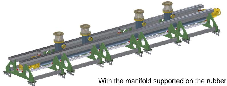
stops of the supported on the rubbe stops of the support frames the whole assembly can now be positioned longitudinally, i.e. So that the first port aligns with the first rebunching cavity.
