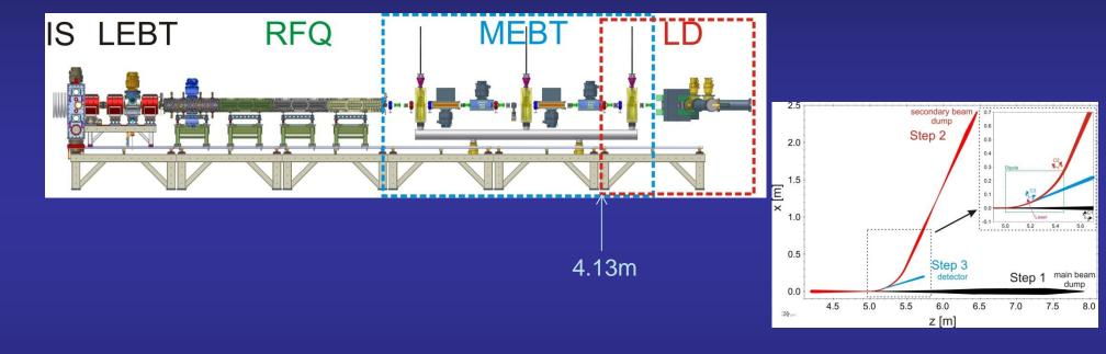
Particle distribution from the MEBT simulation at z=4.13m is used as input to the laser diagnostics lattice simulation.
