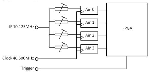
Use an RF source at 10.125MHz, with a splitter and variable attenuation to test the acquisition and FPGA processing. Ensure signals are no greater than 2V peak-to-peak. The clock source is a TTL signal, as is the trigger.
