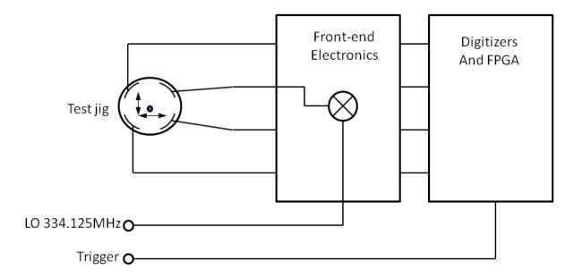
The test-jig uses a movable wire within the BPM, carrying a current with frequency of 324MHz. The LO are trigger are the same as the electronics test.
