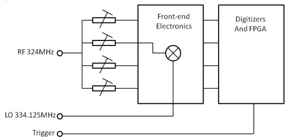
The RF is 324MHz and will emulate the signals from the BPM. The LO should be 10.125MHz different from the RF, either above or below. The LO is either  $31/32 \times RF$ , or  $33/32 \times RF$ .
