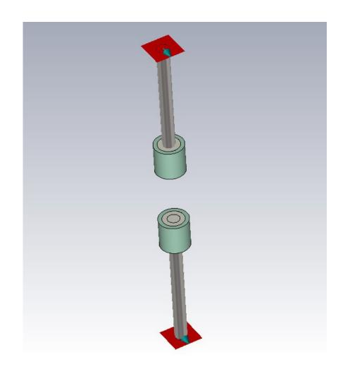
Based on commercially available Alumina tube and weldable N-type feedthrough.
