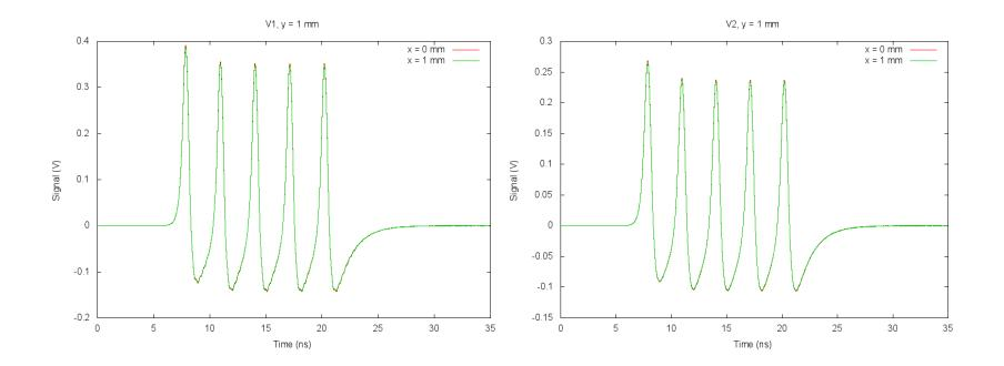
Horizontal offset produces <1% change in vertical signals.
