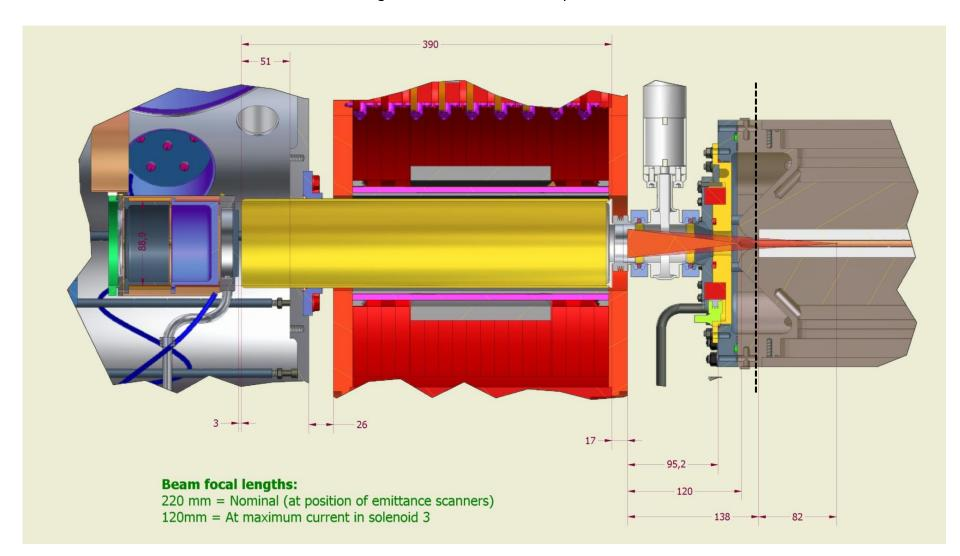
**Position 2:** Beam pipe section 3 fully retracted from the drift vessel.
