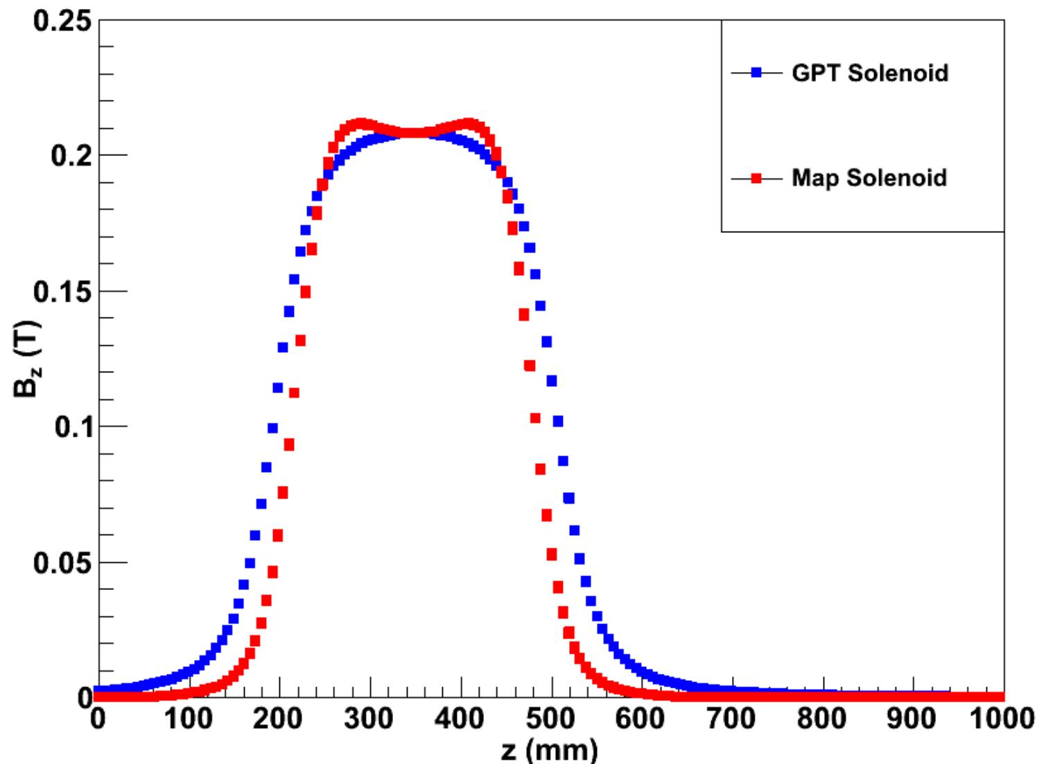
Comparison of GPT solenoid (top) and field map (bottom) for  $I_c = 150$  A (using larger beam radius of 6 mm to clearly see focusing effect)
