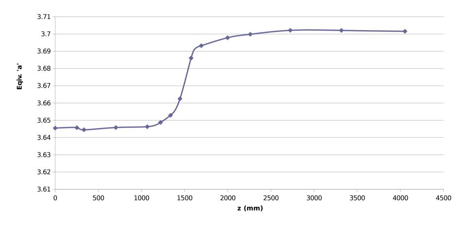
The equivalent shift of the vane tip is  $<60\mu m!$
