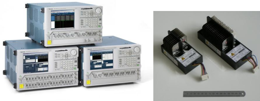
Figure 10: Timing electronics (left) and MOSFET switches (right) for the beam choppers.
