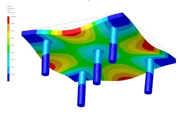
Can use Inventor to help us analyse minimum plate thickness required to give reasonable deformation and stress.
