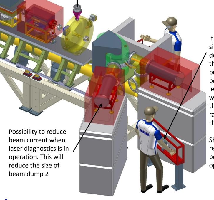
If optics allow could site camera low down in the lee of the two concrete pillars supporting the beam dumps with lead shielding. This will help to protect the camera from the radiation caused by the beam dumps.
