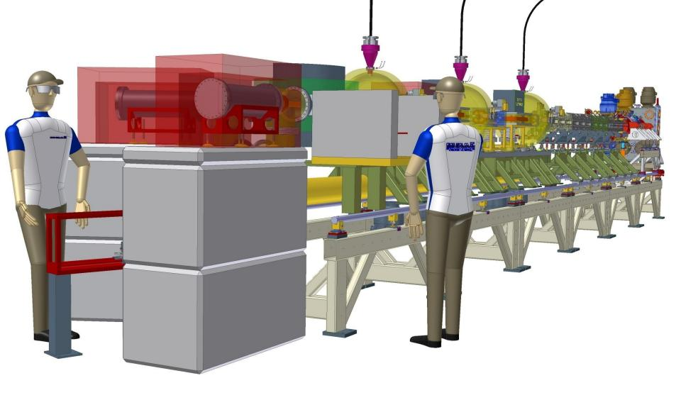
Breadboard shown is 900mm x 600mm. Shielding is 100mm thick lead, both protecting laser from the emitted gamma rays and protecting people from the laser light. Roof and front cover not shown for clarity but may not need such thick shielding.
