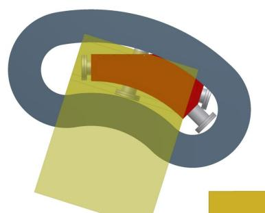
Redrawn coils to match the 2D version shown in CS-PDemi005.dwg and altered the vessel to match the 480mm radius of the central path. Now both vessel and coils share a common axis.
