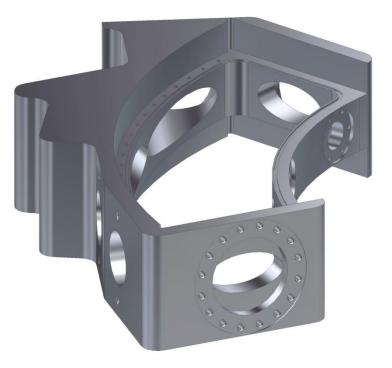
This design is version 7. All previous designs were based on welded fabrications. This design is based on machining from a solid billet which offers several advantages.
