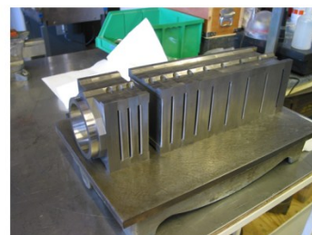
Welded Assembly of Tantalum-Clad-Tungsten Plates. Ready for the last weld.
