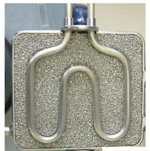
High purity al foam to boost thermal Conductivity.
