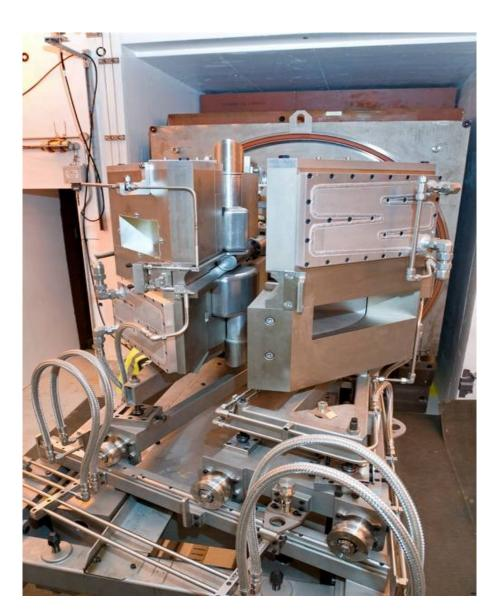
The ISIS TS2 TRAM with the reflector open in maintenance mode and the target and cryogenic moderators revealed.
