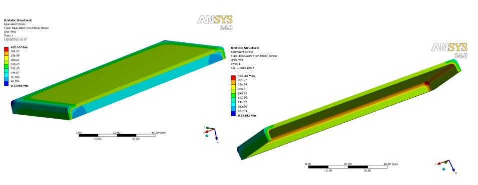
Tantalum is stretched over tungsten due to differential thermal expansion Peak stress of 432MPa in 'rounded' corners, reaching yield stress over large sections too.
