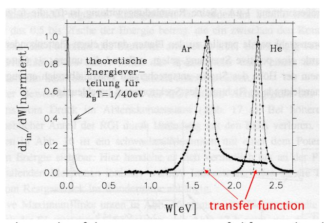
The results of the measurements proofed for He, that the gained ion energy spectra are given by the transfer function and the thermal energy only.
