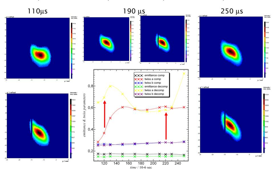
Effect of increased residual gas pressure on beam transport (nominal: 8\*10<sup>-6</sup> hPa and additional Xenon +7\*10<sup>-6</sup> hPa)
