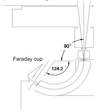
$$W_{particle} = \frac{q \cdot U_{spectrometer}}{2 \cdot \ln \frac{r_{out}}{r_{in}}} = 1.233 \cdot q \cdot U_{spectrometer}$$
