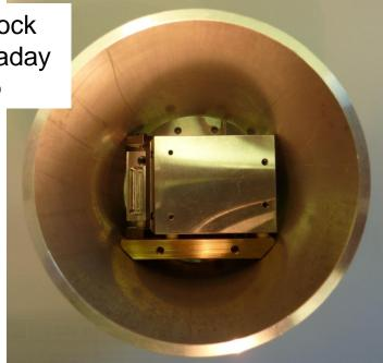
One of the design goals was to make the RGIS4 from available materials. This has resulted in a the mix of materials used, e.g. a brass back plate and an aluminium outer tube.
