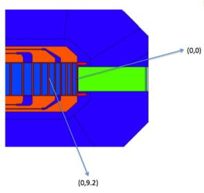
This is the centre of the shielding cylinders i.e where the beamlines are pointing
