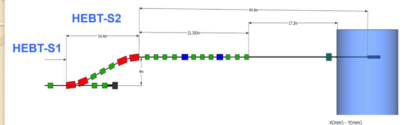
**HEBT-S1:** 100 m long (collimation system + space for additional cryo-modules)
