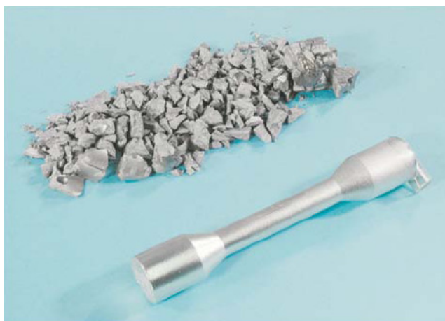
Figure 1.6 Total disintegration of a tin test piece after prolonged exposure to temperatures ca 255 K.[37]
