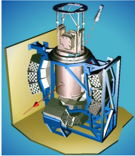
Figure 2.17 PEARL-HiPr instrument with the Paris-Edinburgh cell, in which the Paris-Edinburgh cell is mounted onto a Tomkinson flange and lowered into a vacuum tank.[49] The red arrow indicates the path of the neutrons through the instrument. Diffracted intensities can be collected by two banks of detectors; transverse geometry was used in this study. Longitudinal mode (detectors situated at 20^\circ < 2\theta < 40^\circ and 100^\circ < 2\theta < 120^\circ ) can also be employed to access a wider section of reciprocal space, although resolution is compromised.
